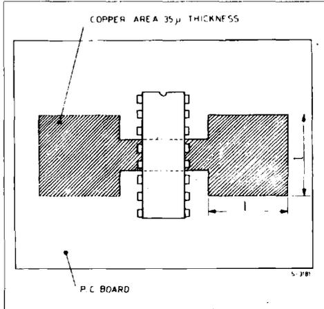
**Figure 16 :** Maximum Dissipable Power and Junction to Ambient Thermal Resistance vs. Side "α".
