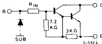
ULN2074B :  $R_{\text{IN}} = 350 \Omega$
