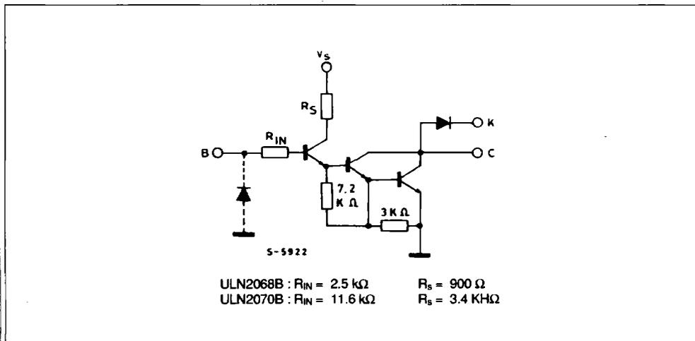
**ELECTRICAL CHARACTERISTICS** ( $V_s = 5\text{ V}$  for ULN2068B,  $V_s = 12\text{ V}$  for ULN2070B,  $T_{amb} = 25\text{ }^\circ\text{C}$  unless otherwise specified)
