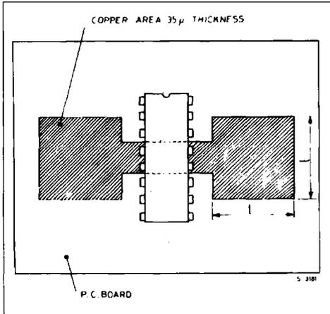
During soldering the pins temperature must not exceed  $260\ ^\circ\text{C}$  and the soldering time must not be longer than 12 seconds.
