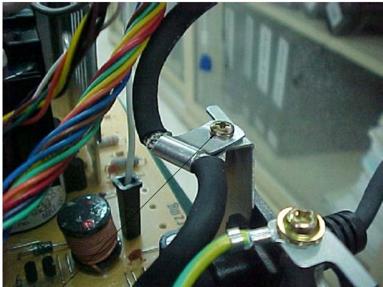
**USE SCREW TO FIX SIGNAL CABLE WITH REAR BKT**
