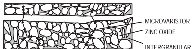
Figure 14. MOV Cross Section
