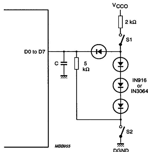
Fig.7 Load circuit for timing measurement; data outputs (FOEN = LOW).
