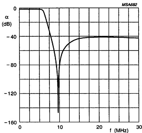
Fig.13 Frequency response for filter shown in Fig.12.
