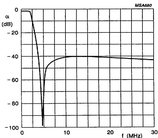
Fig.17 Frequency response for filter shown in Fig.16.
