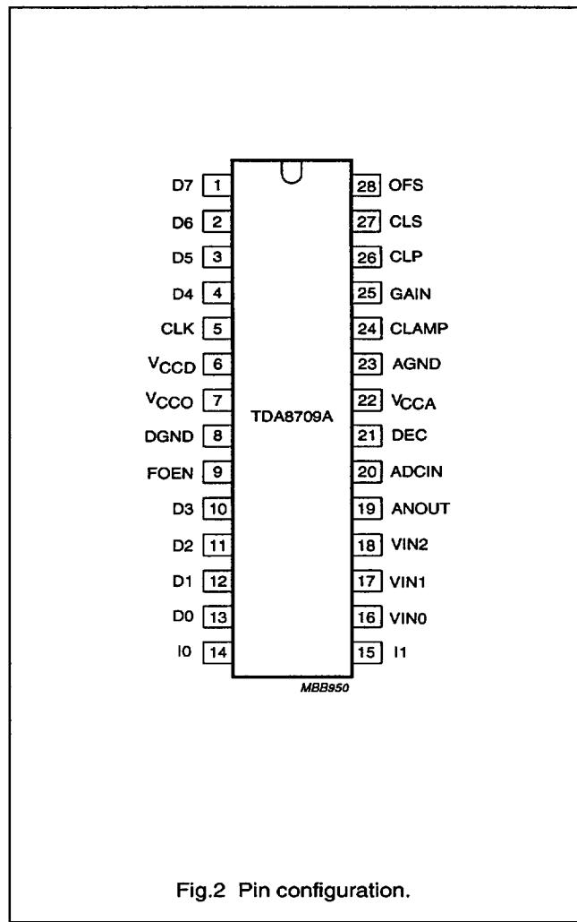
Fig.2 Pin configuration.
