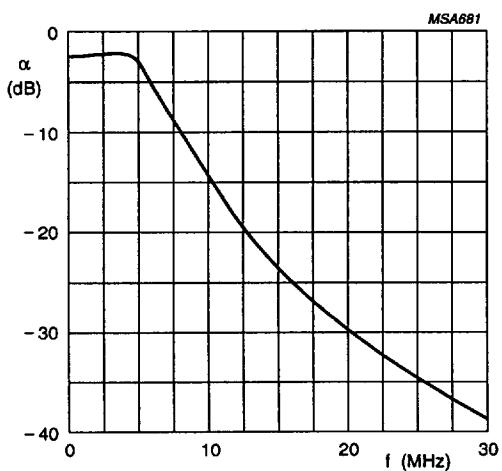
Fig.15 Frequency response for filter shown in Fig.14.
