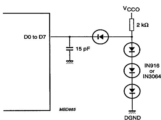
Fig.8 Load circuit for timing measurement; 3-state outputs (FOEN:  $f_i = 1 \text{ MHz}$ ;  $V_{FOEN} = 3 \text{ V}$ ).
