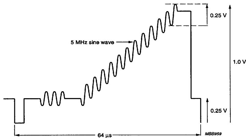
Fig.3 Test signal on the ADCIN pin for differential gain and phase measurements.
