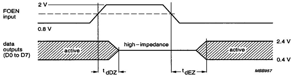
Fig.6 Output format timing diagram.
