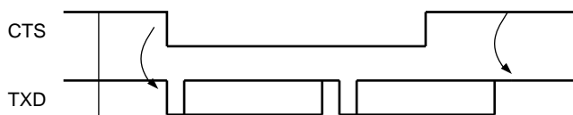
Figure 33-19. Transmitter Behavior when Operating with Hardware Handshaking
