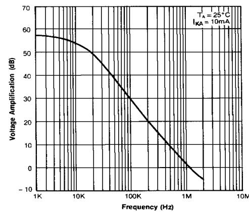
Figure 5. Small Signal Voltage Amplification vs. Frequency
