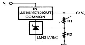
Figure 11. Output Control for Three-Terminal Fixed Regulator
