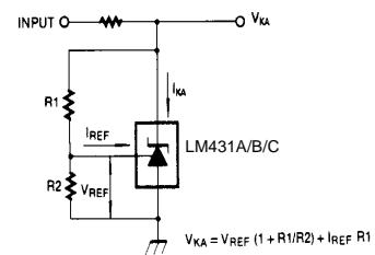
Figure 2. Test Circuit for  $V_{KA} \geq V_{REF}$
